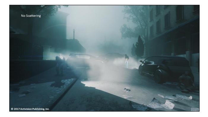
Blocky magnification artifacts can occur due to relative size differences between particles on screen and lightmap texel size resulting in undersampling. Lack of light multi-scattering ( lightmap stores only primary scattering ). Both issues can be improved by lightmap scattering pass.
