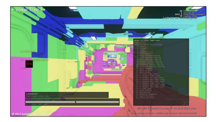
Colors represent amount of lights hitting each pixel. Each voxel stores preculled lights. It is shown here to demonstrate how world space voxels are visualized on surfaces ( not used for actual scene lighting ).
