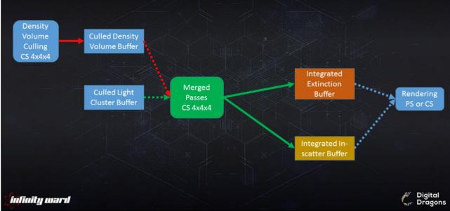
Merge all passes Each pass exists as 'code block' Known VGPR pressure and cycles All input memory read bandwidth optimized Only Write out In-scattering Integral Extinction Integral Need to match kernel size for scalarization Switch all blocks to work with 4x4x4 3D clusters TILE\_MODE\_1D\_THICK In cache, grouped texture Loads and Stores Integral CS required new algorithm to work in 4x4x4 groups Inclusive Prefix Sum Implemented using Lane Swizzles
