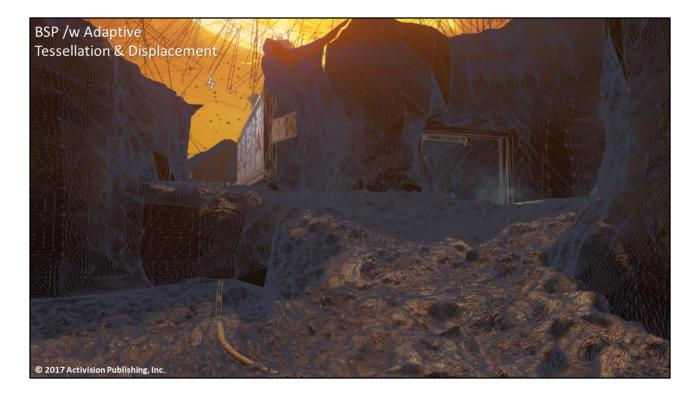
Base BSP with enabled Adaptive Tessellation and Displacement Mapping. Adaptively tessellate based on displacement deltas, distance to camera, patch angle to camera.
