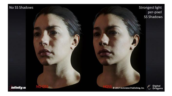
Integrated into F+ Store strongest light source per-pixel Set by artists as key light or derived from runtime computation as max( intensity0...) Perform a single trace in key light direction
