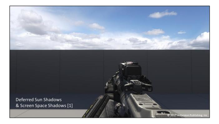
Screen Space Shadow Do a depth buffer raytrace in direction of the light source Deferred pass for Sun Only Optimized for view model ( depth bounds / stencil test ) Works well if run on whole scene
