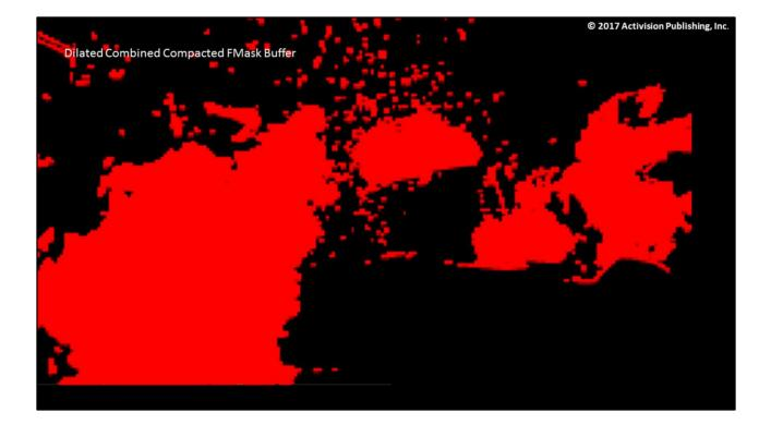
Compacted FMASK Fmask Color > 0 || Fmask Alpha > 0 Packed into 16 bit buffer – 16 bool values per pixel
