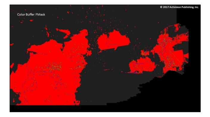
Notice geometric edges marked with multipe samples Gray -> 1 sample / Cmask touched for blending Blue / Green /-> 2 / 3 samples passing rasterizer due to depth intersections Red -> 4 samples due to full resolution rendering or depth intersection hitting all subsamples
