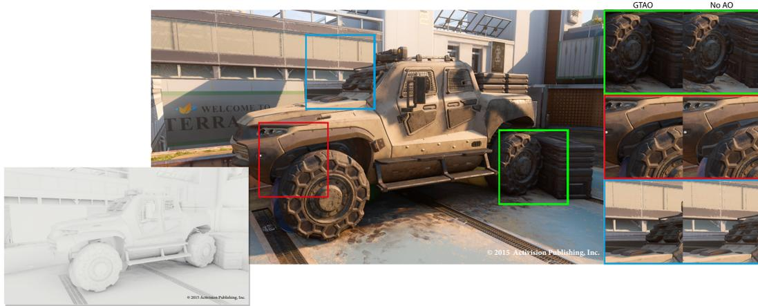
**Figure 1:** Example frame rendered using our Ground Truth Ambient Occlusion (GTAO). The insets on the right, show comparison of rendering using GTAO and the input radiance, while the inset on the right shows the ambient occlusion layer. Our technique achieves high-quality ambient occlusion matching the ray-traced ground truth, in just 0.5 ms on a PS4 at 1080p.
