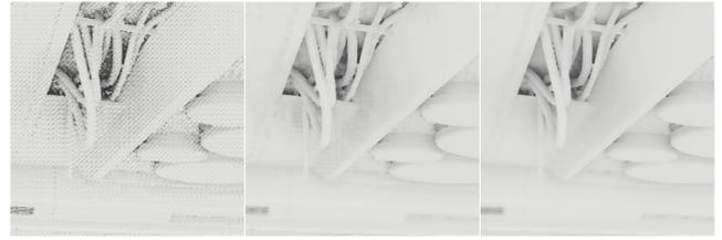
**Figure 3:** Comparison between the samples computed on a single pixel (left), adding the spatial occlusion gathering using a bilateral reconstruction filter (middle), and adding the temporal reprojection using an exponential accumulation buffer (right). In each image we use 1, 16 and 96 effective sample directions per pixel respectively.
