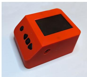
**Figure 9:** Complete device in a 3d-printed enclosure.
