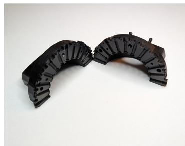
**Figure 5:** The main dome of Reflectometer 2.0, machined in aluminum and anodized in black to reduce stray light. Radial tunnels leading to slots housing sensors and LEDs are visible. Two halves are joined together with screws and positioning pins are used to ensure alignment.
