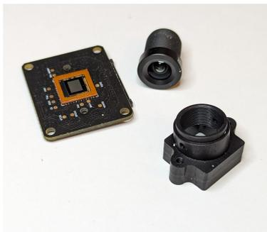
**Figure 7:** Custom camera sensor board, custom angled mount and an off-shelf M12 lens allows for alignment of the focus plane with the sample.
