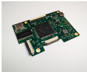
**Figure 8:** Main PCB of Reflectometer 2.0, with STM32H7 microcontroller in the center, memory chip and SD card slot on the left and various peripherals on the right. Connector on the top is used to attach the screen, the one on the bottom connects to the camera board. Flexible PCB with the sensors and LEDs connects to the one on the left.
