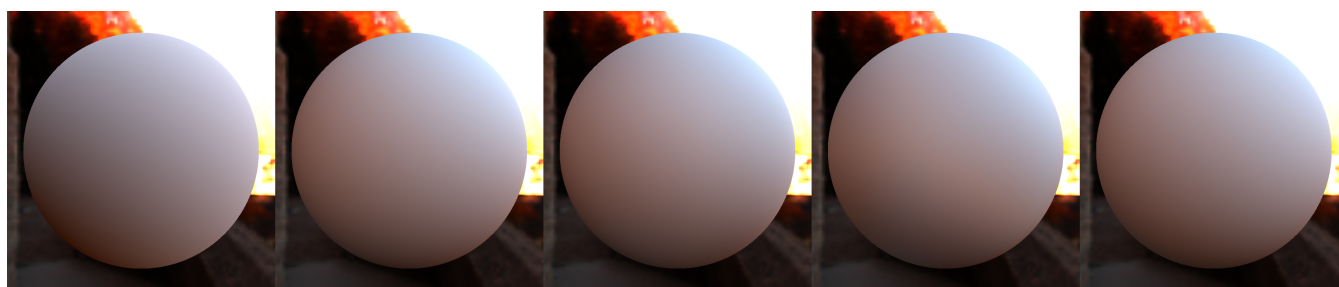
Figure 1: Diffuse irradiance reconstructed using (left to right): 2nd order Spherical Harmonics, 3rd order Spherical Harmonics Ambient Dice (our method) using the RBF variant, Ambient Dice (our method) using the YCoCg variant, importance sampling (reference)
