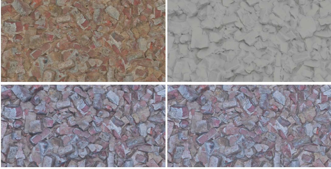
Figure 14: Brick rubble in shadow, clockwise from top-left: Diffuse albedo only, raw material surface occlusion values, render with no material surface occlusion, render with material surface occlusion.
