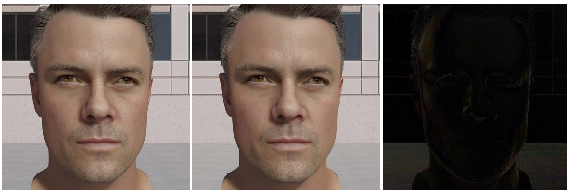
Figure 35: Example of new Multiscattering Diffuse BRDF on skin. Left is Lambertian diffuse, middle is Multiscattering diffuse, right is amplified difference. Notice Lambert diffuse exhibits an unnatural darkening of the face along the silhouette, while Multiscattering diffuse avoids this issue.
